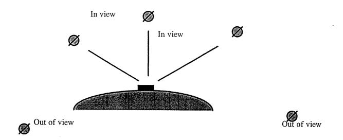
Your unit's location in relation to the position of these four satellites is then used to determine your actual position over the earth.
