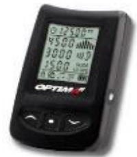
Audible warning device (altimeter), mounted in helmet.
