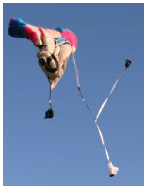
Cutaway main canopy and its deployment bag on the left hooked-up to the reserve's pilot chute, bridle and free-bag on the right.
