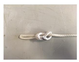
A figure 8 knot may also be used if a 50mm reduction is required.
