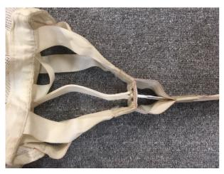
When the kill line is shorter than 50mm, the larks head knot will impact the guide grommet during drogue release. This will cause damage to both the kill line and the guide grommet. Even if the kill line is short, the drogue will still function as designed, but a longer trap door will be experienced and slower deployment may occur.
