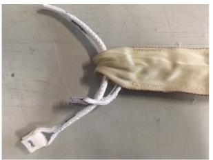
Once the soft link has been installed the bag attachment soft link is to pass through the end of both the soft link and outer bridle.
