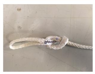
If the kill line has a length of 130mm or more, install an overhand knot just above the base loop in the kill line. A single overhand knot will reduce the length of the kill line approximately 30mm.
