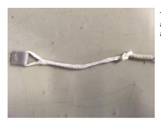
To lengthen the kill line a soft link can be installed at the lower end. This will increase the length by approximately 100mm.
