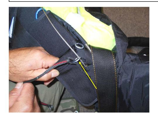
Pass the Ripcord cable through the mini ring of the RSL.
