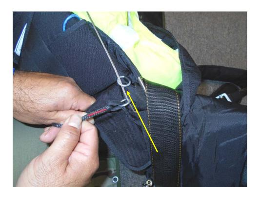
Pass the Ripcord cable through the mini ring on the *Wings* container.
