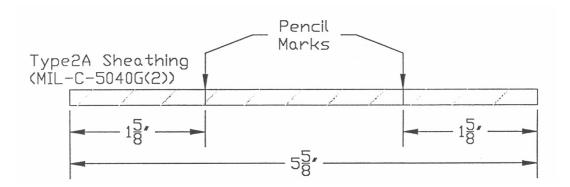
Step 2: Fold the Type2A Sheathing at both 1-5/8" (39mm) marks with the marks to the outside of the fold; creating a 3-layer section of Type2A Sheathing as shown in the figure. It is critical to the finished length of the closing loop that the marks be located at the exact centre of the fold.
