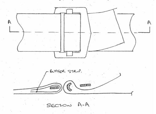
alternatively where there is insufficient space to follow the simple procedure above, the manufacturer a Rigger 'B' must incorporate a webbing buffer into the webbing securing the Chest Strap Adaptor by unpicking the stitching securing the Chest Strap and afterwards fixing the adaptor in place by duplicating the original stitching.
