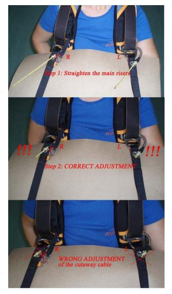
3. The left main riser must be released 15 mm (½ inch) prior/before the right one with the RSL.
