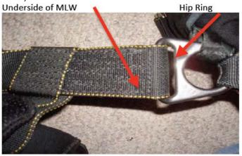
5. Rotate Hip ring and leg pad 90 degrees downward as to expose the top of the ring to the inside of the folded bottom end of the MLW webbing, as shown below.
