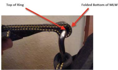
6. Move the hip ring back and forth (side to side) and rotate inside the webbing, while pressing the top of the ring through the webbing. If a needle strike is present, the rough spot on the top of the webbing bar of the ring will catch or snag on the TYPE 12 buffer on the inside of the TYPE 7 MLW. This will feel like a rough spot(s) on the top of the bar and cause a rough or snagging feel.
