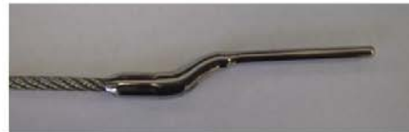
Pic. 4 B Pressed pin – bent, hexagonal press
