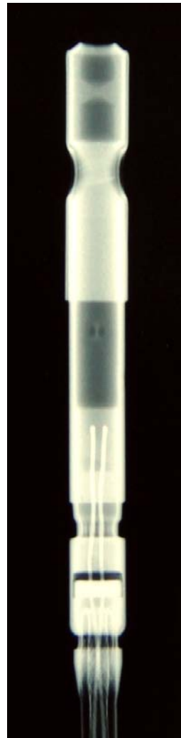
Cutter of unit S/N 11258 after jump 288 (Part Number 9582006)
