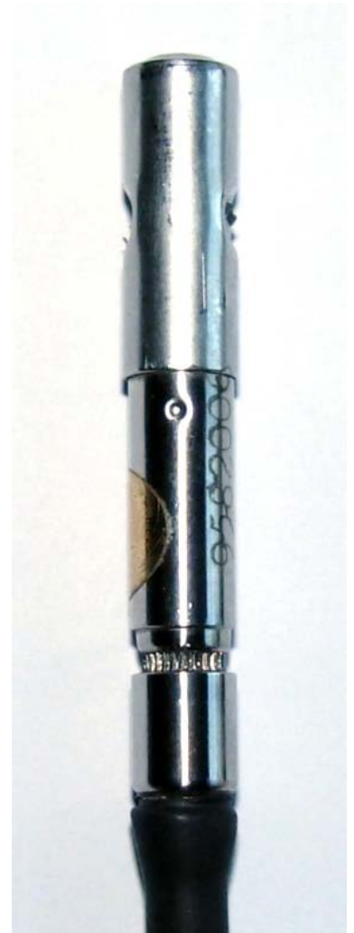
Cutter of unit S/N 11258 after jump 288 (Part Number 9582006)
