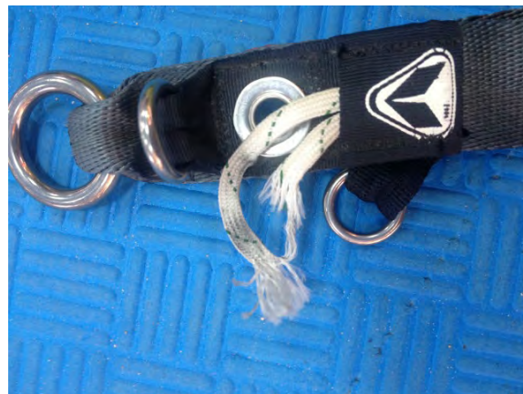
DAMAGED, PARTIALLY CUT
