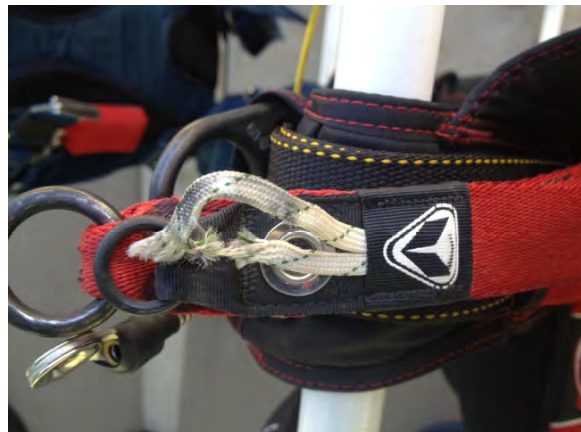
DAMAGED, PARTIALLY CUT
