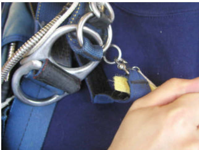
picture 1 (wrong, Velcro between the RSL )
