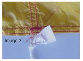
Image 2: Damage at one of the 'B' line attachment points
