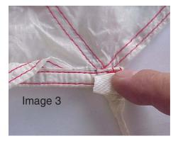
Image 3: Pulling back the line attachment loop reveals the 28 stitch tack in the leading edge.
