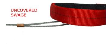
After removing the heat shrink, check for broken filaments. If any are found, replace the ripcord immediately.
