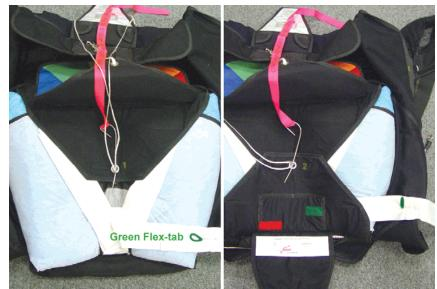
**3.** Attach the RED Skyhook lanyard to flap #2 by folding the stiffened section of the lanyard in half, and inserting it completely into the RED pocket on the flap. You may have to open the pocket a little with a pencil before inserting the flex-tab.
