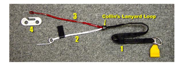
4. The Skyhook itself, which is sewn to the reserve pilot chute bridle. (Because the RSL Lanyard, Collins' Lanyard, and Skyhook Lanyard are all part of one integrated system, pulling the yellow tab on the RSL snap shackle inactivates all three.)
