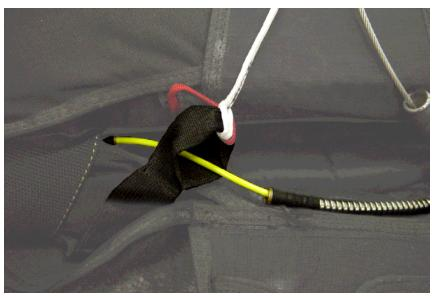
Make sure the left hand (exposed) yellow breakaway cable passes through the Collins' Lanyard loop at the end of the RSL. The Skyhook should not be used without a Collins' lanyard.
