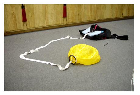
2. S-fold the 8-foot section of freebag bridle (up to the Green flex-tab) under pilot chute kicker flap #1, in the normal manner. Close flap #2, and secure with the reserve closing loop and temporary pin. Make sure the remaining bridle exits the closed kicker flaps to the wearer's LEFT (Right in photos) of the #2 (upper) flap, with the flex-tab side up.
