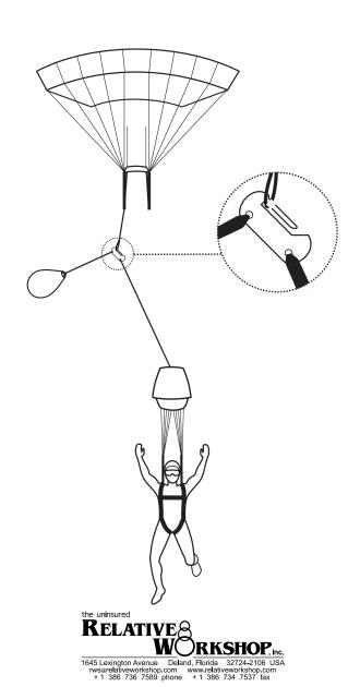
A standard RSL does one thing. It pulls the reserve ripcord pin automatically after a breakaway. The Skyhook RSL does this, and then goes two steps further.
