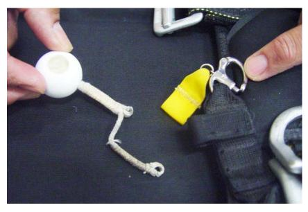
This picture shows the crystal ball after it has been removed. Ensure that the RSL release tab remains intact.
