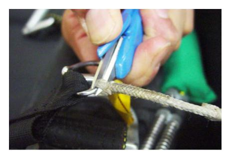
Second, cut the remaining dacron line attaching the Crystal Ball to the RSL shackle.
