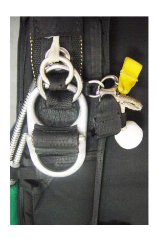
View of a standard Sigma RSL with the Crystal Ball.
