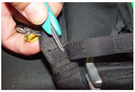
Remove the velcro tab from the RSL. This tab is intended to hold the Crystal Ball in place.
