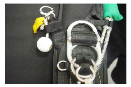
To remove the crystal ball, first cut the short piece of 600lb dacron line connecting the Crystal Ball to the RSL shackle.
