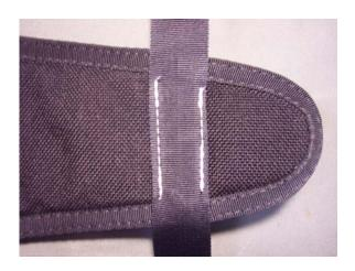
7. Cut the Type 3 tape to leave approximately 1" tails. Roll the tails to hide any exposed edges and sew the tails to the binding tape.
