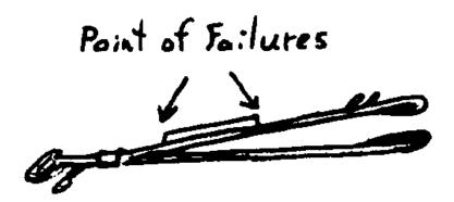
**BACKGROUND:** Over the last four months Strong Enterprises has received notification of several main risers failing. The manufacturing dates on these risers span several years. All failures have occurred at the toggle pocket location on the rear riser. SEE SKETCH: Because neither age nor number of jumps is a reliable gauge, it is not possible to determine ahead of time when a failure might occur.
