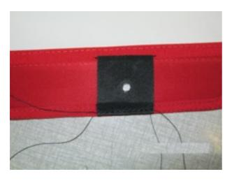
Fold under excess material and sew on
