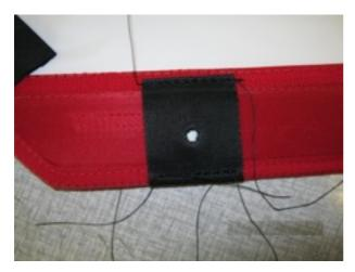
Fold under excess material and sew it on
