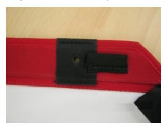
Re-attach cutter keeper according to Airtec Riggers Manual
