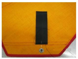
Place 12 cm Type XII piece onto outside of flap, line up with grommet centre and sew it on
