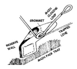
There are a number of other brands of equipment manufactured this way, some with the grommet facing the reserve wall, some with the grommet facing the main bag that could be susceptible to this.
