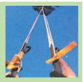
be on half brakes on one side and full drive on the other. If the toggle fires at a late stage in the deployment, then the result is likely to be a good canopy that is turning, but that can be corrected by releasing the other toggle. However, if the brake fire happens early on, then the canopy has much more time to become uneven during the deployment itself, leading to twists as is happening in the photo below.
