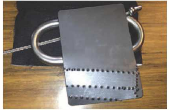
Image 3: Showing most likely possible snag position between the metal handle and plastic stiffener
