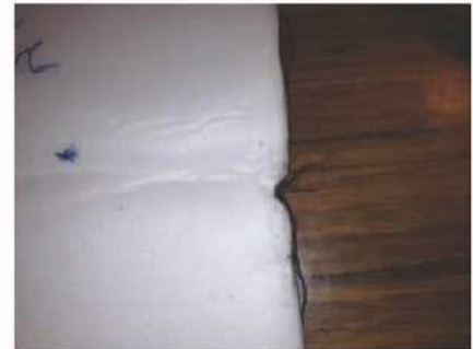
Image 4: Showing indentation on foam corresponding to swage position indicated in image 3
