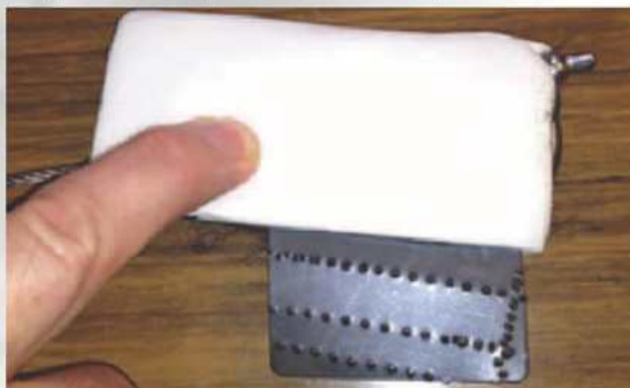
Image 2: Cover removed & showing the swaged end of the cable in the wrong position
