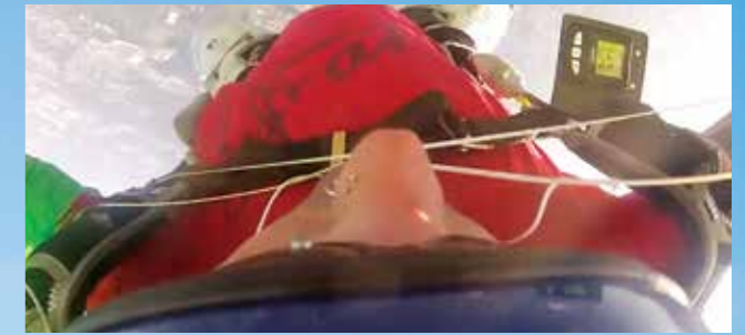
Upper Jumper in Wrap: Unsafe to cutaway – clear or contain lines and fabric
