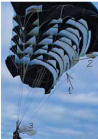
1. The original GLH SYSTEMS two parts ultra low drag risers. Third riser was added for the Accuracy application.
